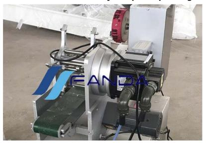
5. Because the cutting speed is changeable, so it can meet the cutting requirement on the 100kg/h soap production line, 300-800kg/h soap production line and 1000-2000kg/h soap production line.
